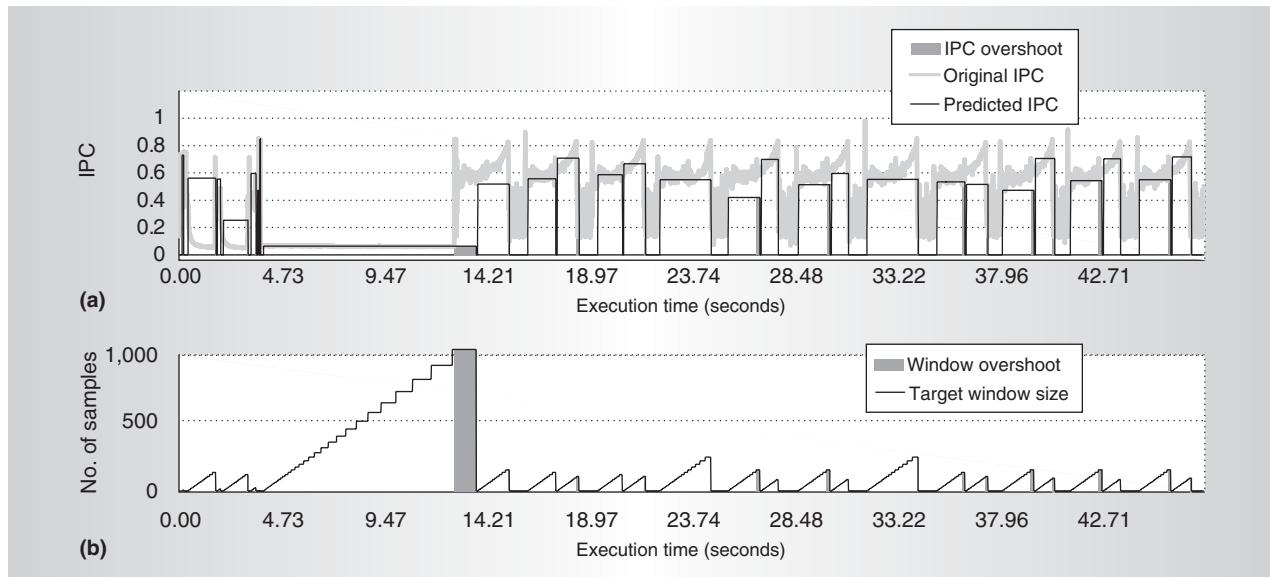
Figure 1. Duration prediction for ammp with FXby8: original and predicted IPC (a) and target window size (b).
