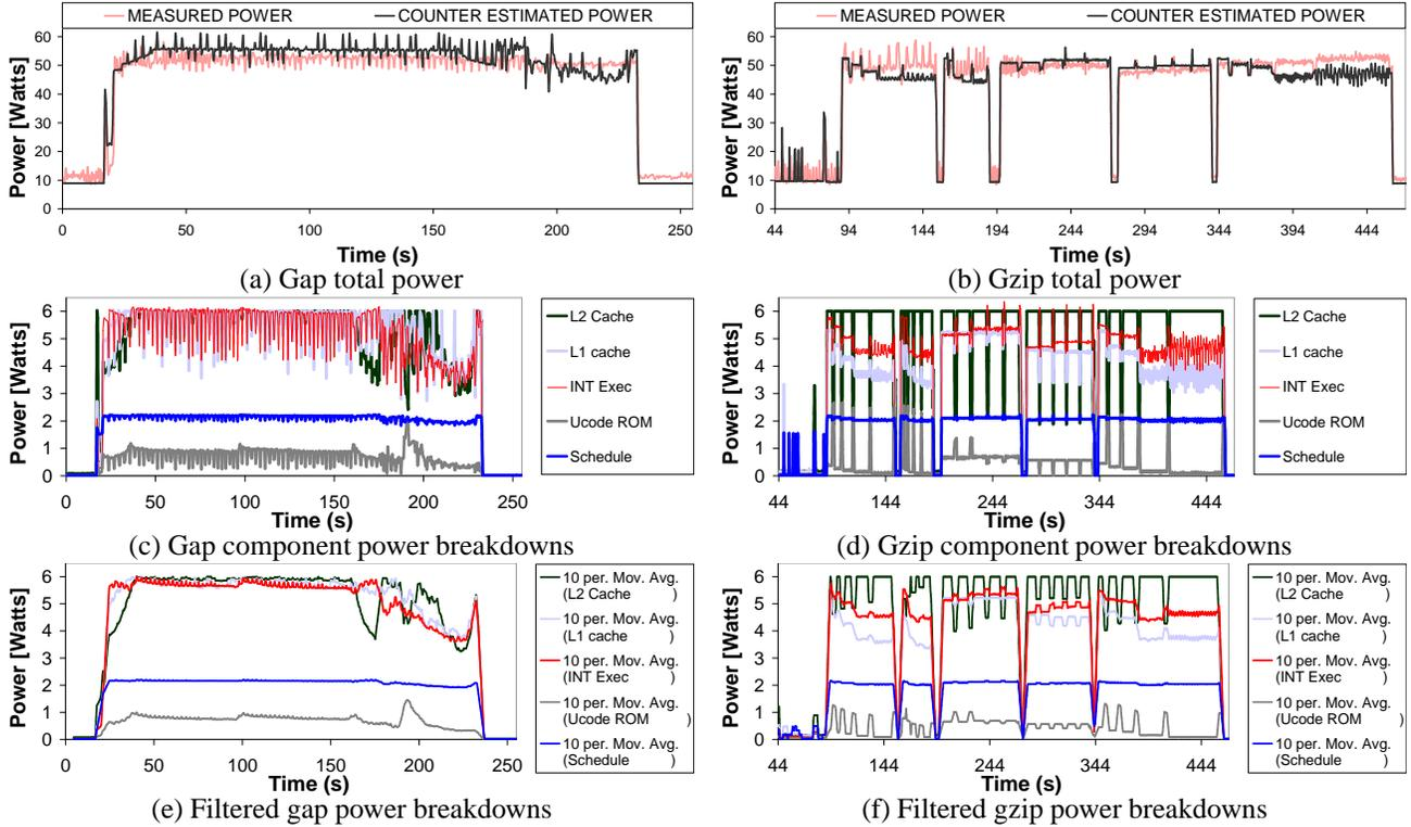
**Figure 2. Total and component-wise power traces for gap and gzip.**
