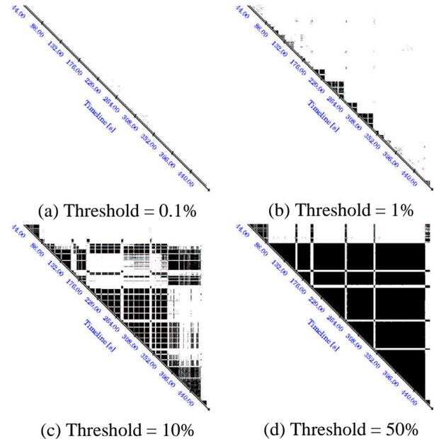
**Figure 5. Grouping matrices for gzip with respect to different threshold values.**
