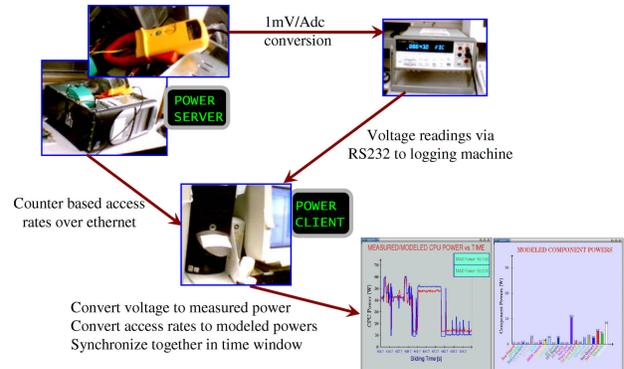
**Figure 1. Power measurement and component power estimation setup.**
