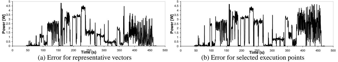
**Figure 12. Absolute error in total power estimates reconstructed from representative vectors and selected execution points.**
